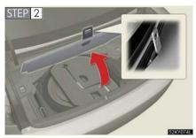
Secure the panel using the hook provided.
