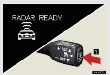
Selecting vehicle-to-vehicle distance control mode
