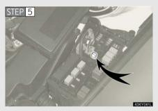
Remove the fuse with the pullout tool.
