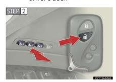
While the desired button ("1", "2" or "3") press on the wireless remote control until the signal beeps.
