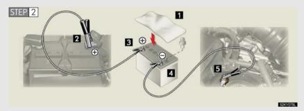
Connecting the jumper cables.
