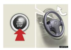
When the "FNGINE START STOP" switch is turned OFF, the steering wheel returns to its stowed position by moving up and away to enable easier driver entry and exit.
