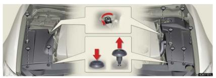
Installing the clips
