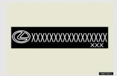
These labels are attached to the vehicle to reduce vehicle theft by facilitating the tracing and recovery of parts from stolen vehicles. Do not remove under penalty of law.
