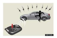
When (() is pushed for longer than about one second, an alarm will sound for about 60 seconds and the vehicle lights will flash to deter any person from trying to break into or damage your vehicle.
