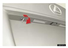
Turn the mechanical key clockwise to open.
