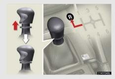
Shift the shift lever into the R position while lifting up the ring section
