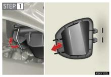
Release the lock and remove the cover.
