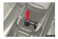
Remove the cup holder insert holding the base part.
