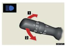
1 With the headlights on, push the lever forward to turn on the high beams.
