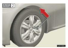
Slightly loosen the wheel nuts (one turn).
