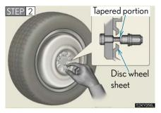
Install the spare tire and loosely tighten each nut by hand to approximately the same amount.
