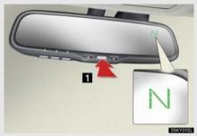
To turn the compass on or off, push "AUTO" for longer than 3 seconds.
