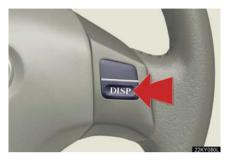
Display items can be switched by pushing the "DISP" switch.
