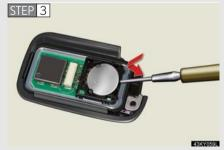
Remove the depleted battery.
