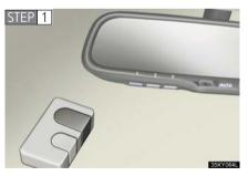
Point the remote control for the device 1 to 3 in. (25 to 75 mm) from the HomeLink® control buttons.
