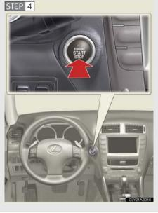
Press the "ENGINE START STOP" switch.
