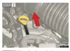
Hold a rag under the end and pull the dipstick out.
