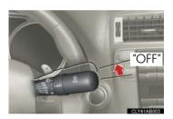
Set the wiper switch to "OFF". If the wiper switch is in "AUTO", the wipers may operate and the wiper blades may be damaged.
