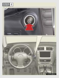
Press the "ENGINE START STOP" switch.
