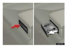
To open, press in and release the rear cup holder on the rear center armrest.
