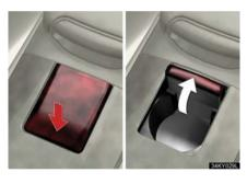
To open, press down and release the front of the cup holder lid.
