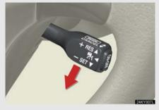
Accelerate or decelerate the vehicle to the desired speed and press the lever down to set.
