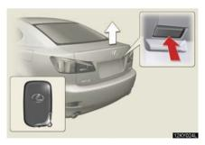
Press the button to unlock the trunk.
