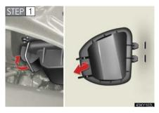
Release the lock and remove the cover.
