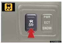
Quickly push and release the button to turn off TRAC.
