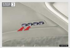
While pushing the "SET" button, push button "1", "2" or "3" until the signal beeps.
