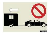
Do not tow the vehicle backwards. Doing so may cause serious damage.
